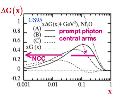
>  $\Delta G$  with NCC at low-x through jet- $\gamma$ ,  $\pi^0$ , e- $\mu$ , open charm.
