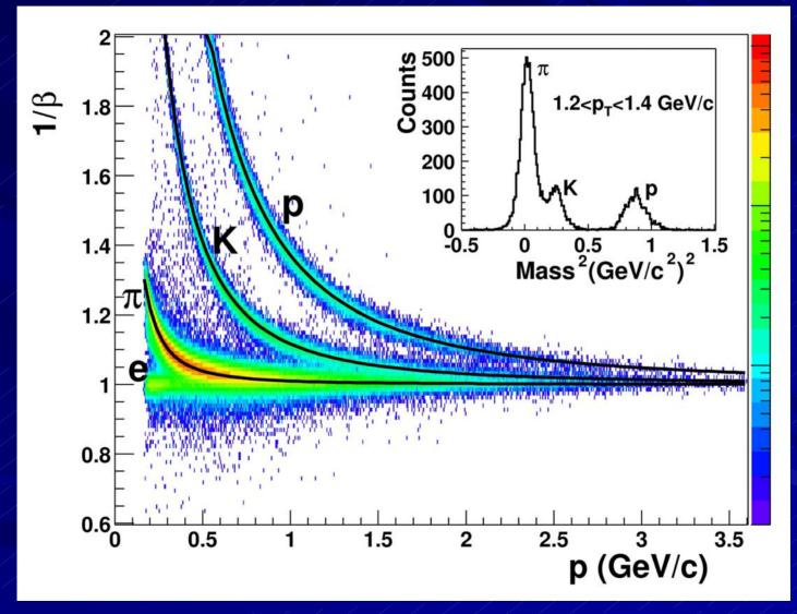
$\pi/K$  separation p~1.6GeV/c, p/(K+ $\pi$ ) p~3GeV/c
